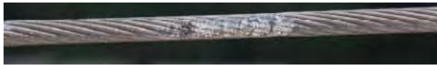
Figure 20 shows one of two adjacent AAC midspan conductor arc melts from galloping
