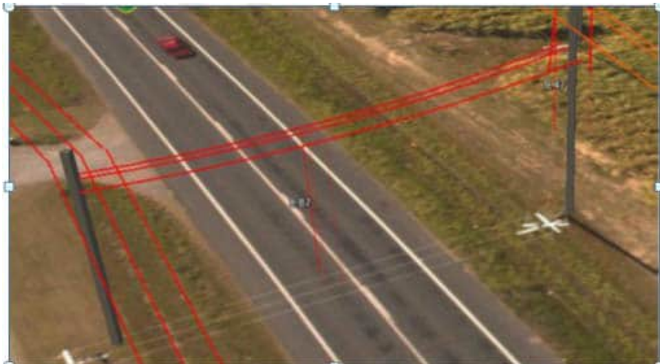
Figure 15: 3D image example of a LiDAR survey identified a line span conductor clearance risk.
