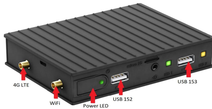
Figure 3: Horizon Power's SGD hardware and port overview 2
