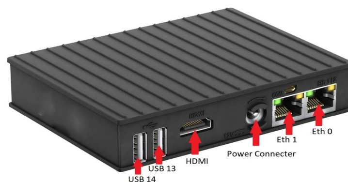
Figure 2: Horizon Power's SGD hardware and port overview 1
